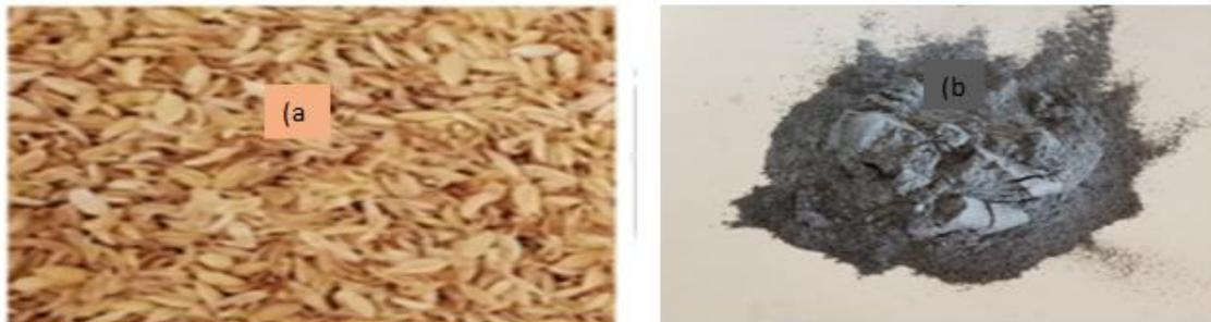
**Fig. 2. Rice husk(a) and rice husk ash obtained after calcination(b)**
