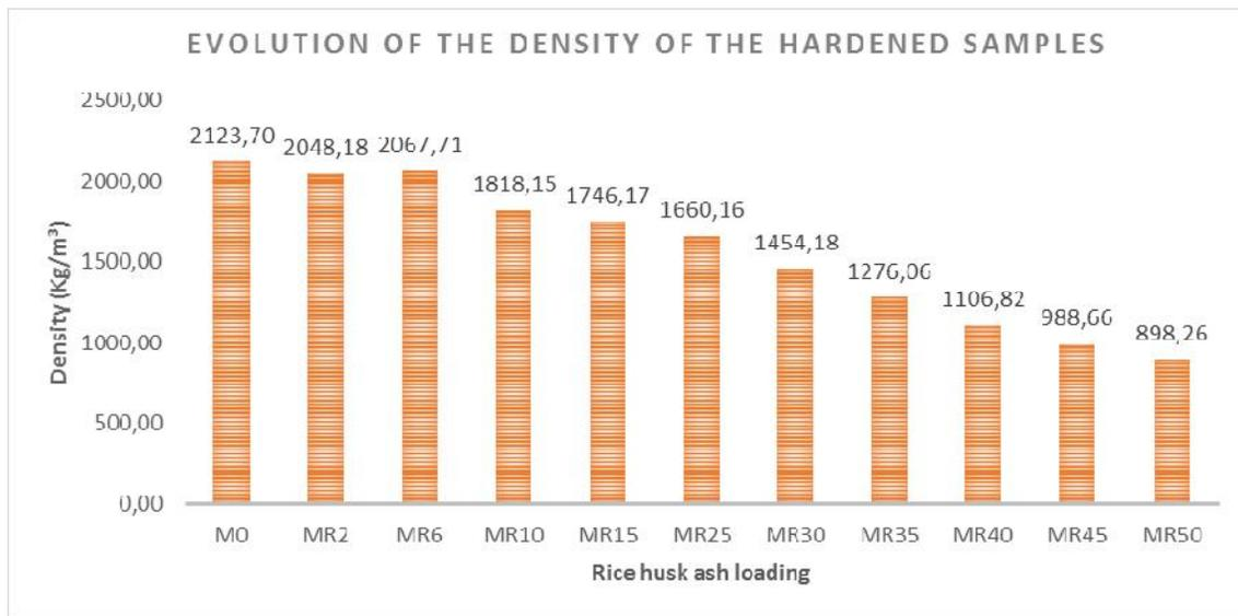
Fig. 9. Density of hardened samples as a function of the rice husk ash loading
