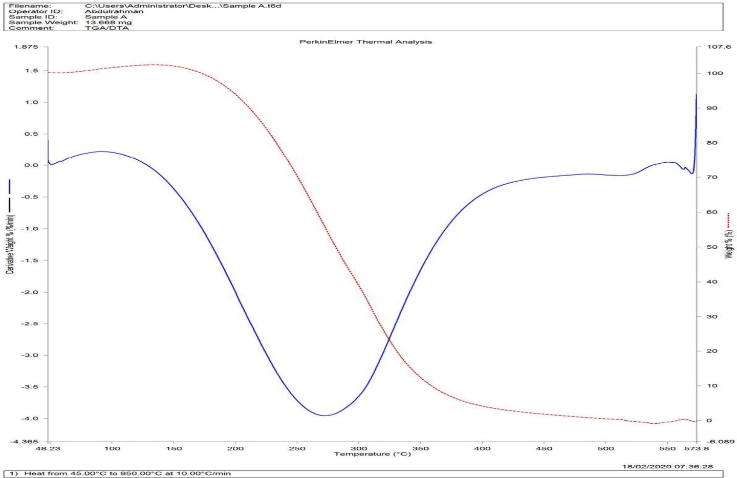
Fig. 6. TGA curve of the rice husk ash
