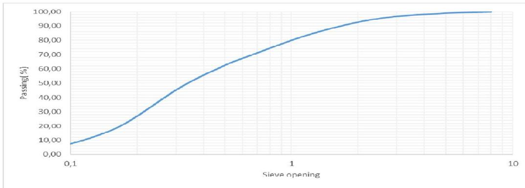
**Fig. 1. Granulometric analysis curve of the sand**
