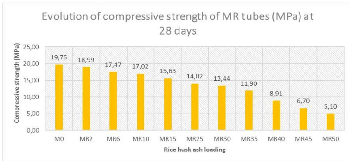
Fig. 10. Compressive strength of MR pieces as a function of rice husk ash loading
