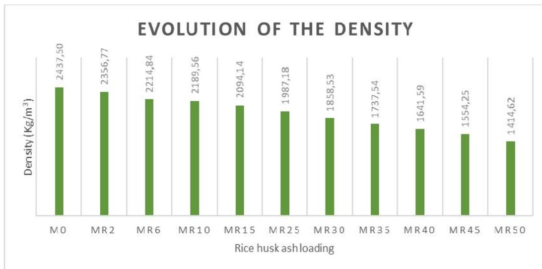
Fig. 8. Density of fresh mortar as a function of the rice husk ash loading
