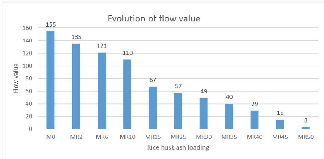
Fig. 7. Evolution of the Flow value as a function of the ash loading
