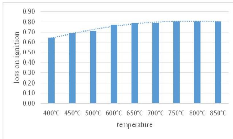
Fig. 4. Evolution of loss on ignition as a function of temperature
