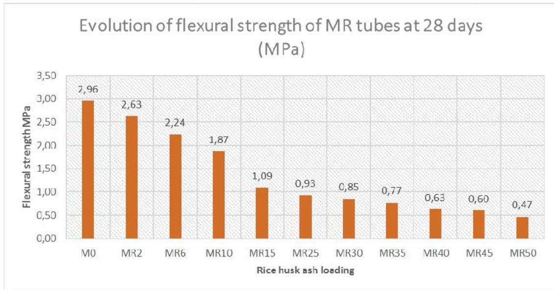
**Fig. 11. Flexural strength of MR tubes as a function of rice husk ash loading**
